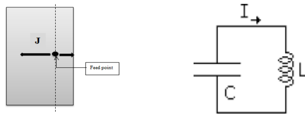
Figure 1: Current distribution of normal patch antenna and equivalent LC circuit.
