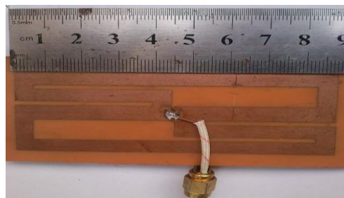
Figure 5: Hardware designed for the proposed antenna.
