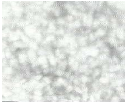
Fig.4: Neutron Radiographic image of fire ricks (Optimal irradiation time 50 min).
